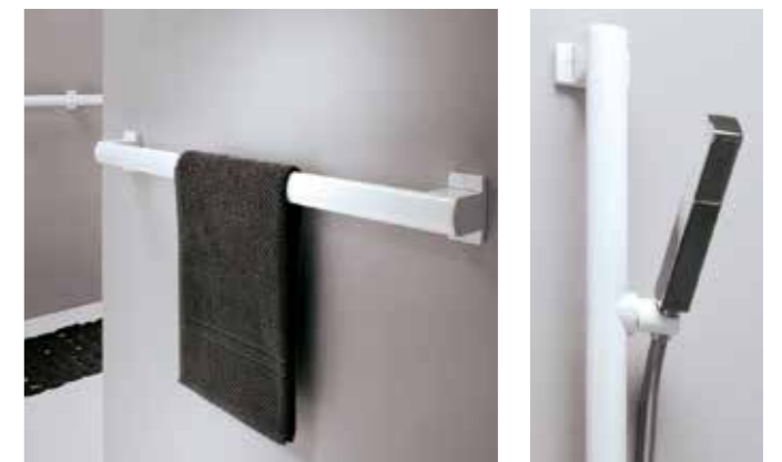
Straight grab bars. Elliptic tube, 38 x 25 mm., white or anthracite grey epoxy-coated or anodized aluminium. White, anthracite grey, mat or bright chrome-plated resin flanges. Concealed fixings.
