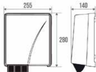
Hair dryer 2100 W. 300 m<sup>3</sup>/h output. Temporizing push button 2,15 mn. The resistance in chlorinated atmosphere.
