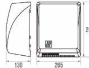
Hand dryer 2600 W. Aluminium cast iron. 300 m<sup>3</sup>/h output. 75 dBA. Vandal-resistant. 3 years warranty.
