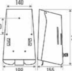
Liquid soap dispenser - aluminium. Capacity 1500 ml. White epoxy-coated aluminium + cataphoretic steel.
