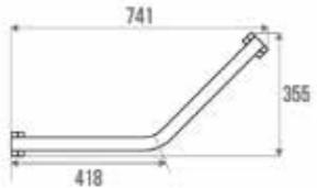
135° angled bar, 2 fixing points, symmetric, 400 x 400 mm.
