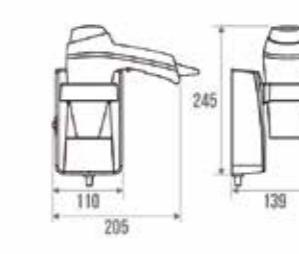
Hair dryer 1400 W. 70-95 m<sup>3</sup>/h. output. Touch-sensitive switch. 3 temperature levels.
