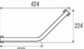
135° angled bar, 2 fixing points, symmetric, 200 x 200 mm.
