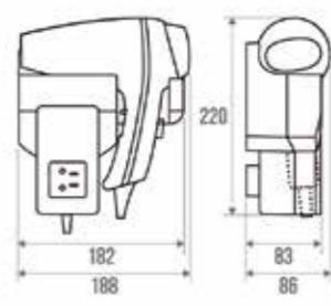
Hair dryer 1400 W. 70-95 m<sup>3</sup>/h. output. Shaver plug. 115/230 V. 3 temperature levels.
